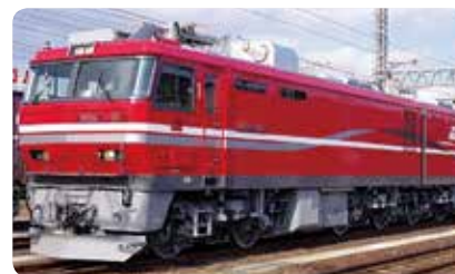
A new EH800 model locomotive for Japan Freight Railway Company (A locomotive designed specifically to run in the Seikan Tunnel sharing it with the Hokkaido Shinkansen)
