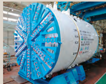
TBM (EPBM type: blue part is the cutterhead)
