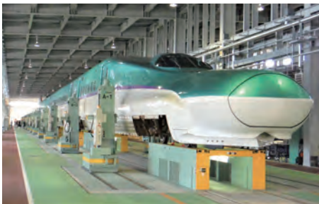
Bogie replacement machine, Hokkaido Shinkansen
